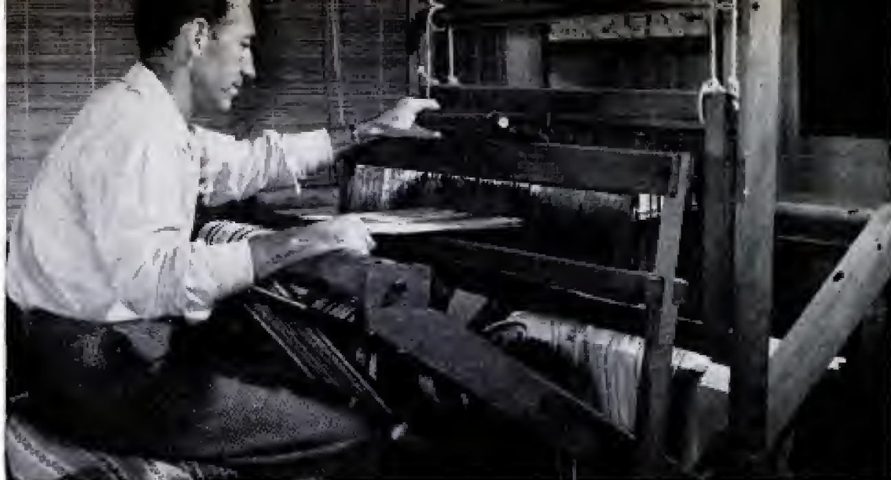
After yarn pattern is set up on loom, each piece of wood is inserted individually and shuttle operated by hand
